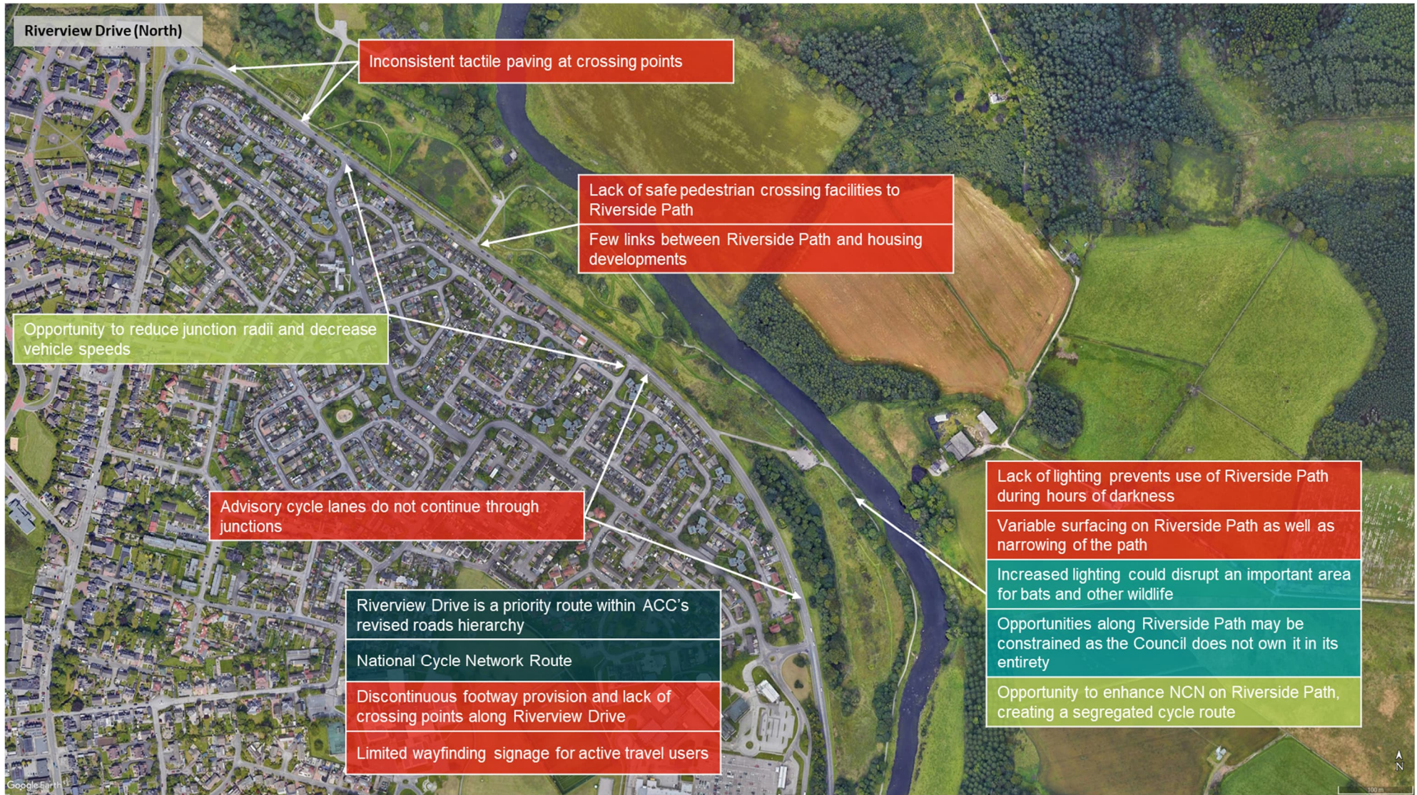
Figure 9.3: Location-Specific Issues on Riverview Drive (North) (Image Source: Google Earth)
