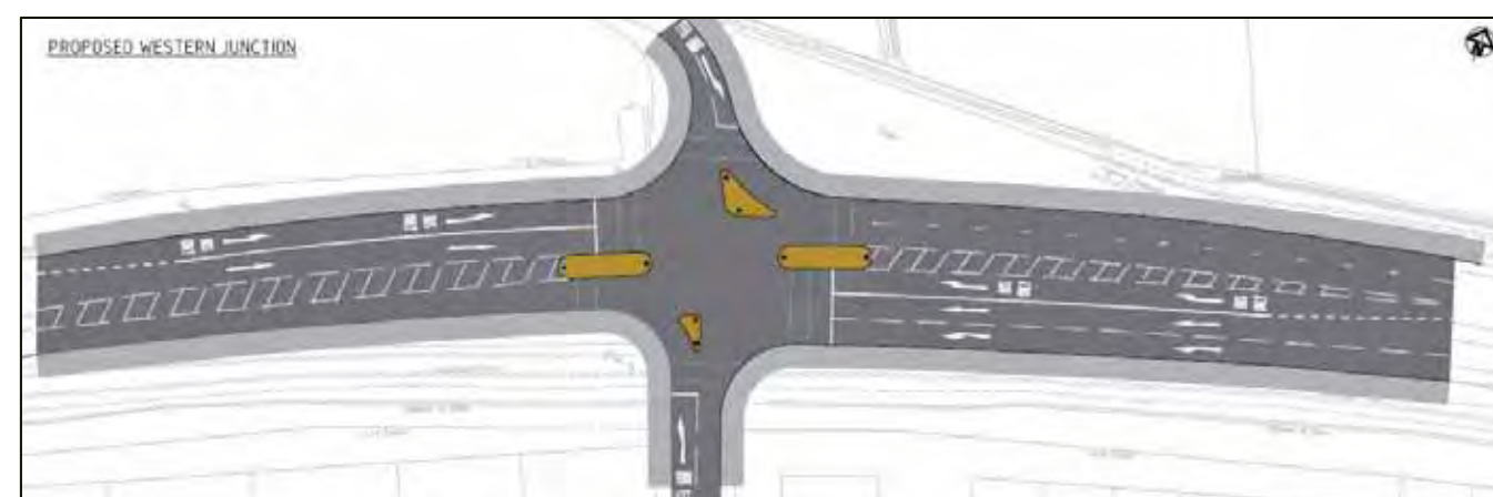
Fig 25 – Western junction – indicative left-in/left-out solution
