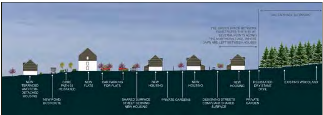
Fig 47 – section 1 - indicative section through the boundary of area A and the woodland to the North.
