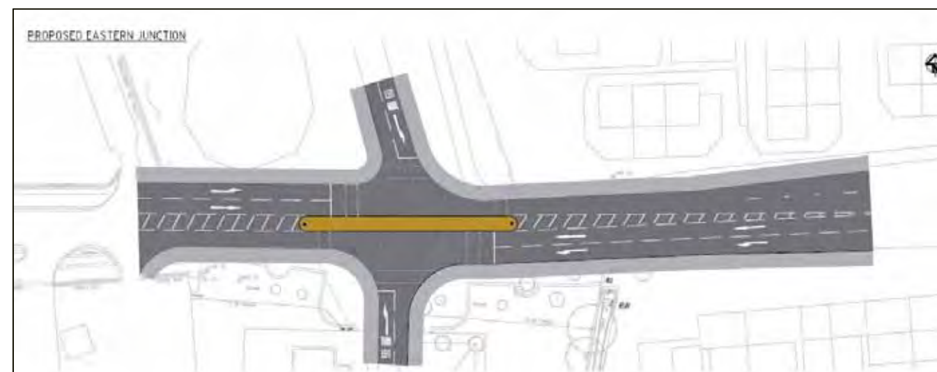
Fig 24 – Eastern Junction – indicative layout – final left-in/left-out solution
