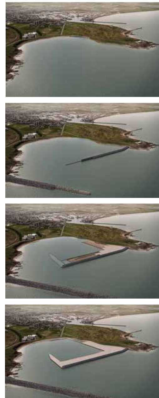
FIGURE 20 Harbour Construction Visualisations up to year 2
