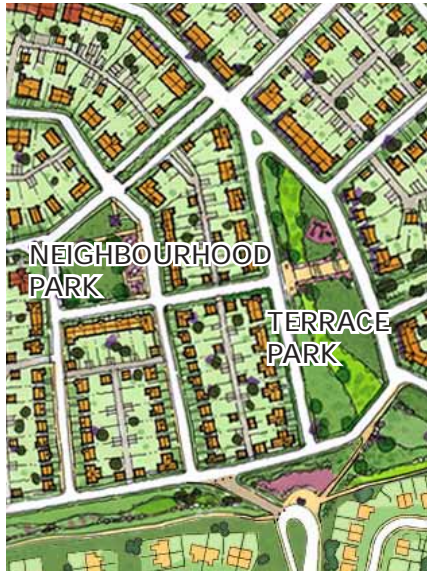
Figure 3.11 The enlarged plan features a terraced park, which incorporates and preserves portions of the existing steep slope and acts as a green buffer between the existing neighbourhoods and the proposed blocks. West of the terraced park, a small neighbourhood park with gardens and garden features provides an intimate address for the surrounding units.
