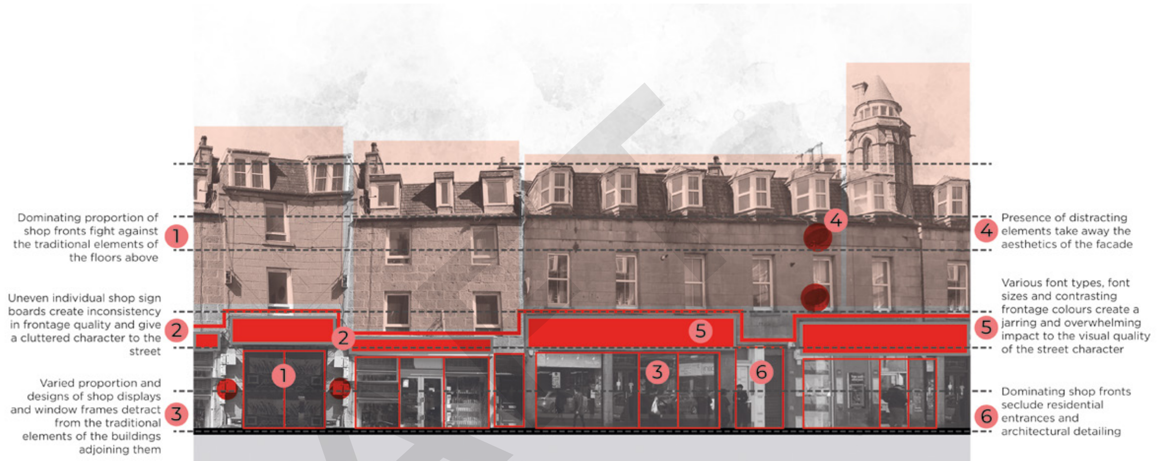
Figure 30 - Inconsistencies in George Street's shop frontage
