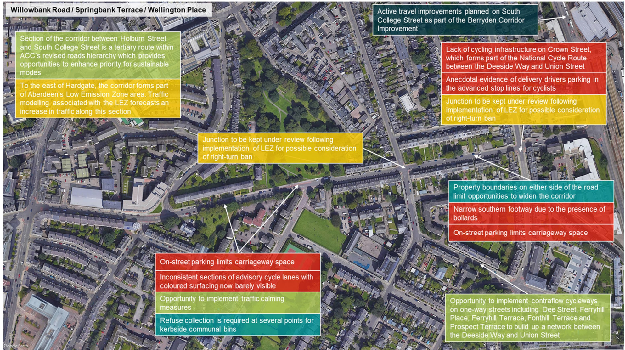
Figure 4.15: Willowbank Road / Springbank Terrace / Wellington Place PICOs (Image Source: Google Earth)
