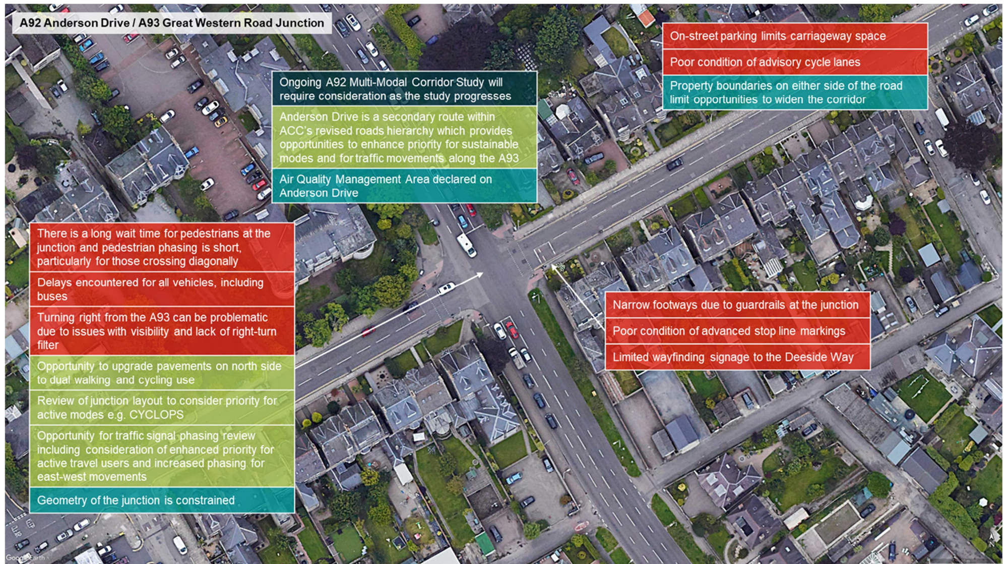
Figure 4.13: A92 Anderson Drive / A93 Great Western Road Junction PICO (Image Source: Google Earth)
