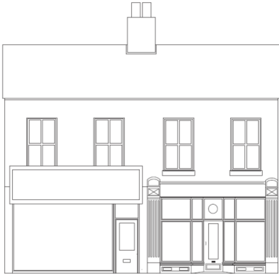
Modern, poorly-designed shopfront with excessive fascia
