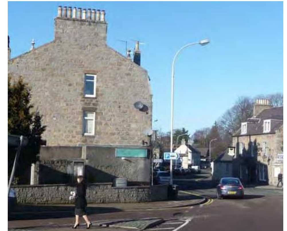
Windows in gables overlooking public space adds to townscape and street security
