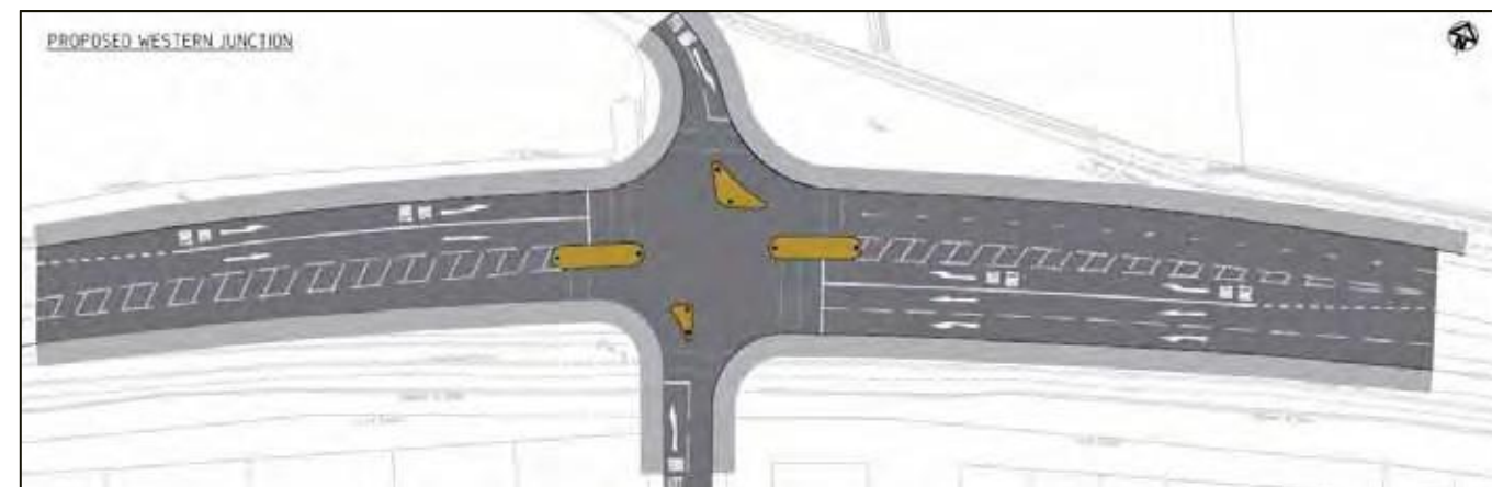
Fig 25 – Western junction – indicative left-in/left-out solution
