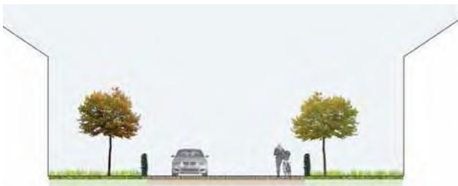
fig. 51: Indicative section: Street Type C. Shared surface.
