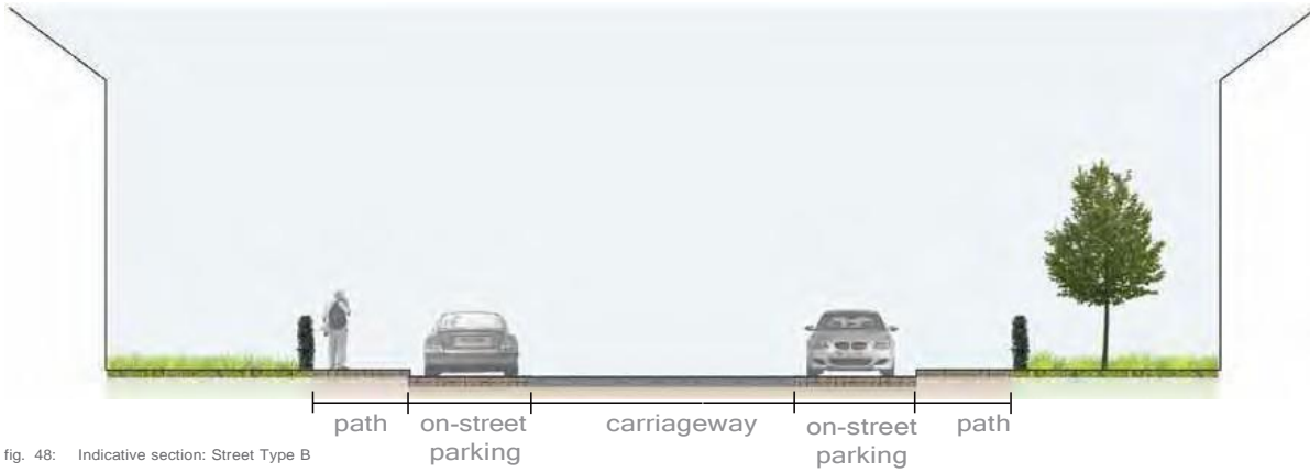
fig. 48: Indicative section: Street Type B
