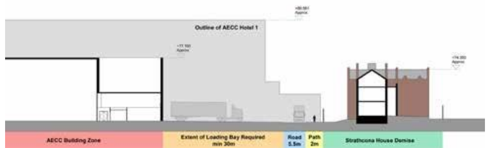
Loading/Service Zone required following swept path analysis
