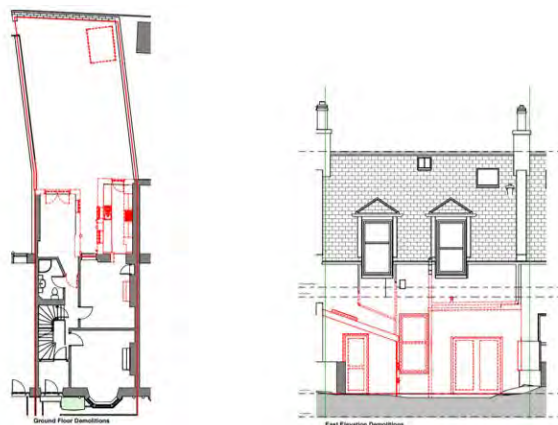
Figure 2: Image showing proposed demolitions to rear (east elevation). All demolitions shown in red.
