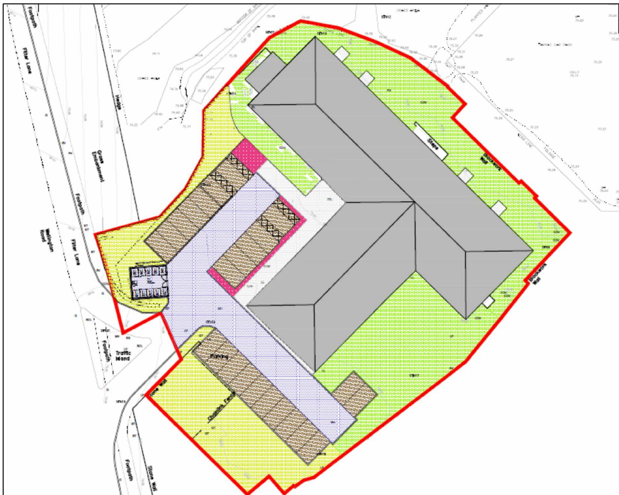
Figure 4: Proposed Site Plan showing that there will be minimal external works required other than to reduce the overall level of hardstanding (Source: Bradley Craig Architects)
