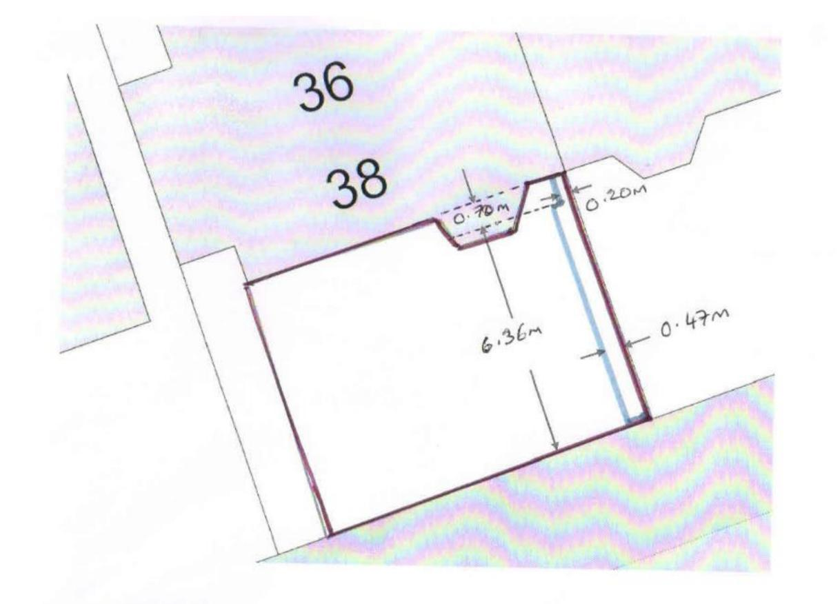
Fence shown in grey. Wooden slated (11 x 15cm deep planks); painted grey. Height: 1.70 metres. Width of of wood: 0.02m. Dimensions, including distance from boundary, shown.
