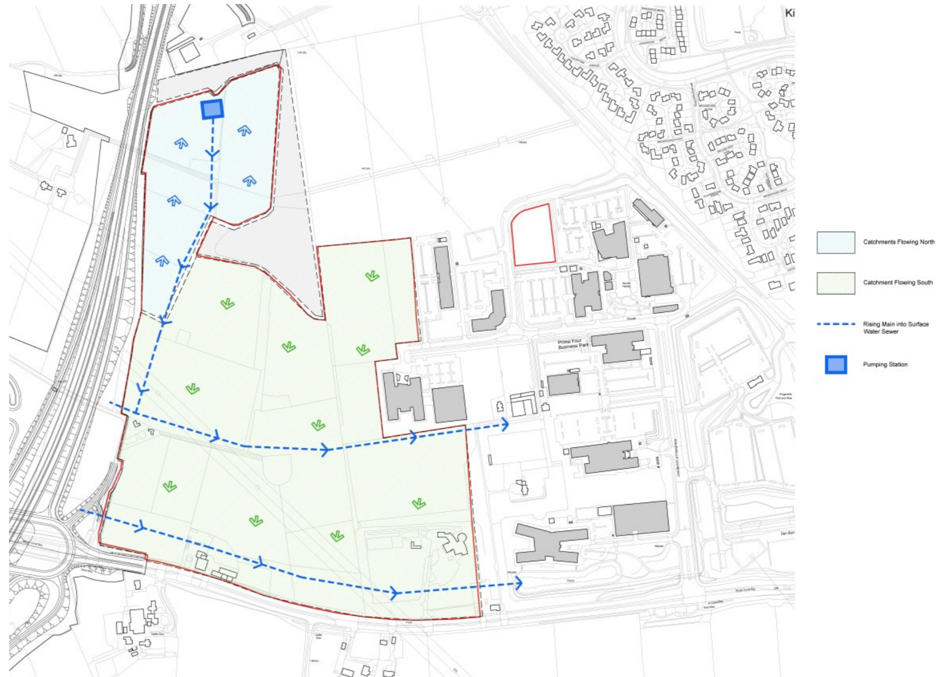
Figure 26: Indicative Drainage Diagrams
