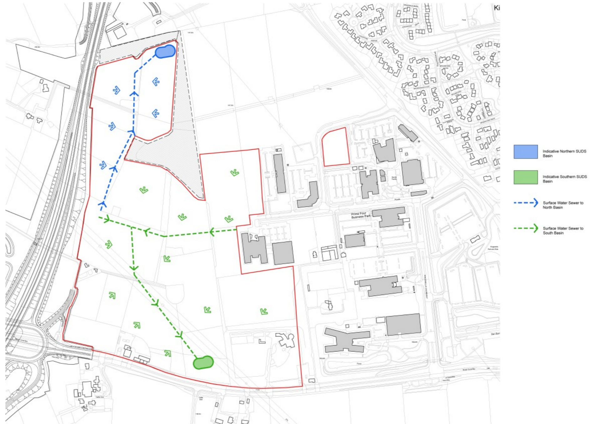
Figure 27: Indicative Drainage Diagrams
