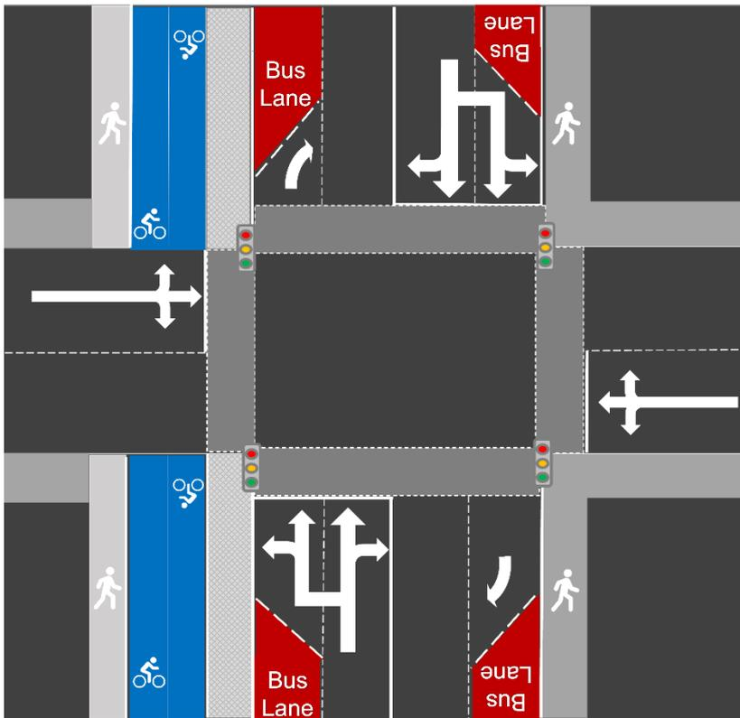
Figure 4.5: Intervention Level 1 – Standard Cycle Lanes - Layout (with 2-way cycle track)
