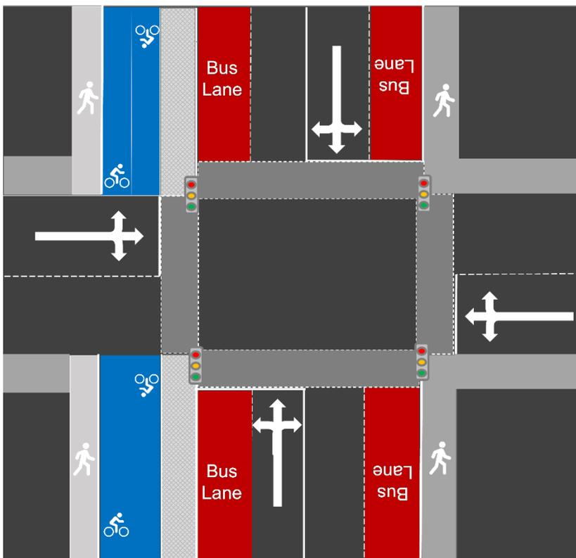
Figure 4.6: Intervention Level 2 – Enhanced Cycle Lanes – Layout (with 2-way cycle track)
