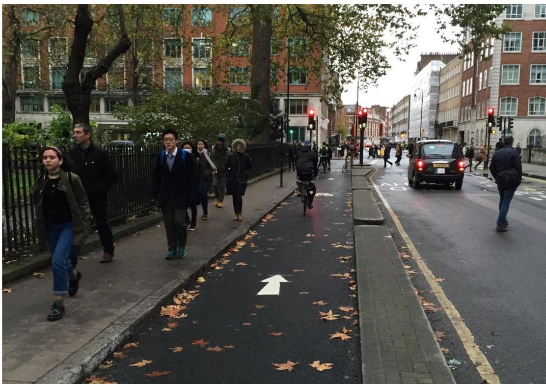
Figure 4.3: With traffic flow - segregated cycle track - Examples
