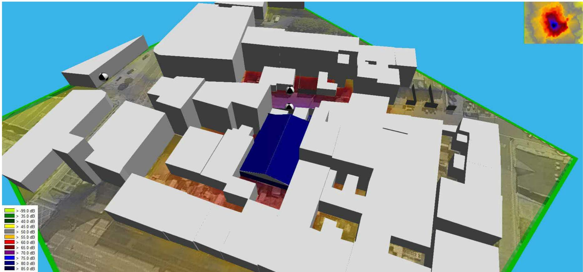
Figure A4.3: 3D Noise Grid with Vertical Grid – Doors Open
