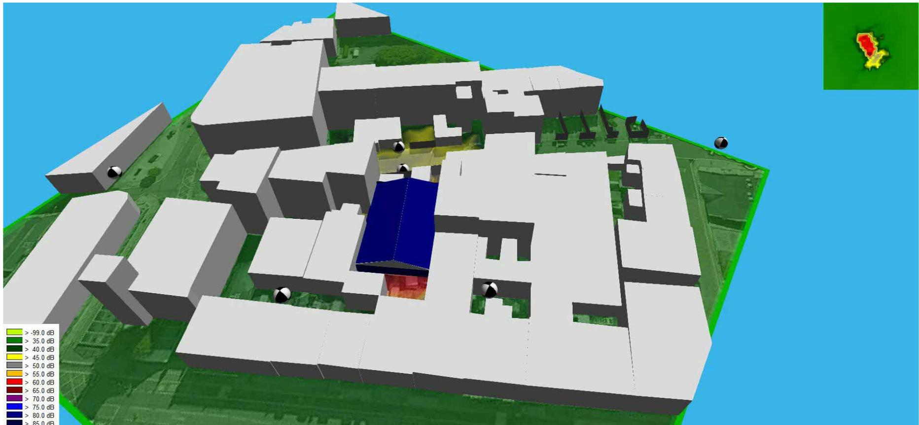
Figure A4.6: 3D Noise Grid with Vertical Grid – Doors Closed
