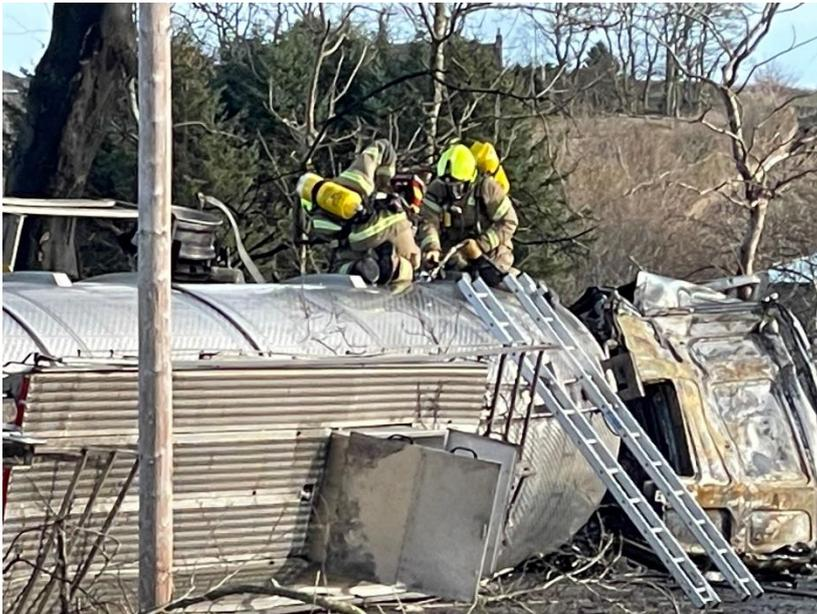
6.4: EPU: Specialist clay putty utilised to stem leak of substance from ruptured tanker. Boom systems and chemical absorption mats/socks used to contain substance from entering drains and open water source.
