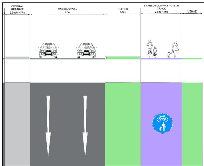
**Figure 9.1 Shared Footway / Cycle Track Cross Section**
