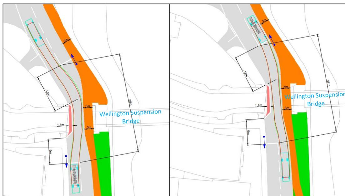
Figure 48. Riverside Drive - Shuttle Working Design Swept Paths
