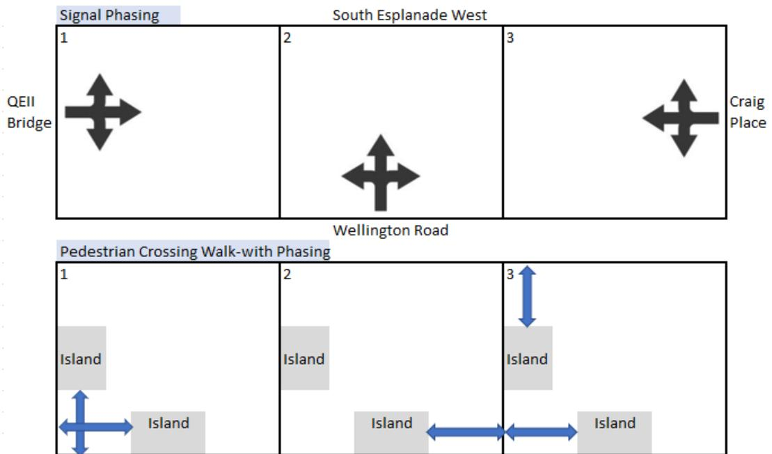
**Figure 38. Southern QE Bridge Concept Junction Phases**
