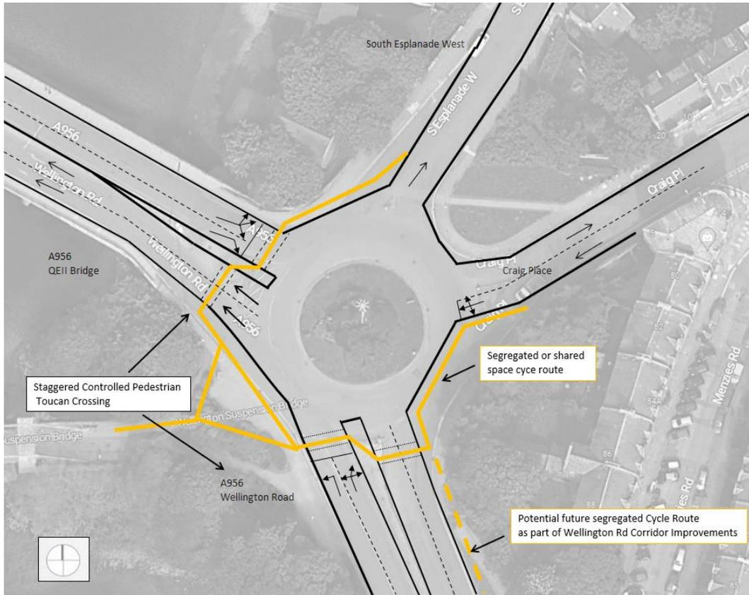
**Figure 37. Southern QE Bridge - High Level Concept Junction Design**
