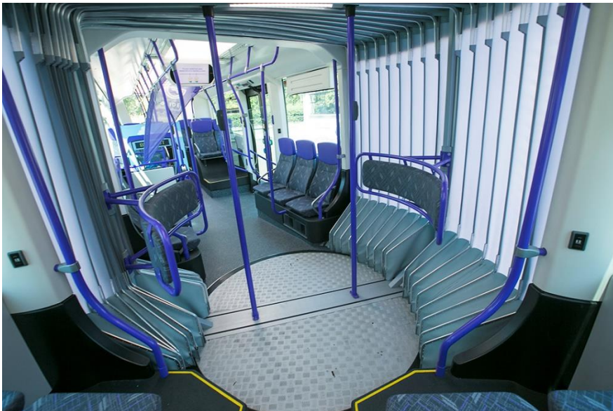
Figure F:5: Belfast Glider tram-style vehicle - interior (Photo courtesy of Translink)
